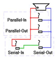
If you have a lot of Floor Monitor needs, you might consider adding an extra couple of serial input connectors (the two existing input connectors on each Floor Monitor will be parallel wiring).
