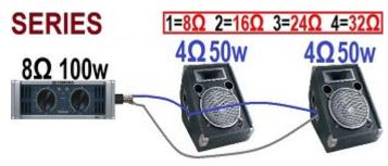
If we connect cabinets using the wiring shown here, then we are making a "series" circuit. With series circuits the resulting ohms becomes the total of all we added. 1=8  $\Omega$  2=16  $\Omega$  3=24  $\Omega$  4=32  $\Omega$ . In this example the Loudspeakers are 4 ohm ones so they add to 8 ohms. That suits the specs on the example 8  $\Omega$  Power Amplifier and so it will deliver 100 watts. The power will always spread across all cabinets, so each loudspeaker will get 50w.
