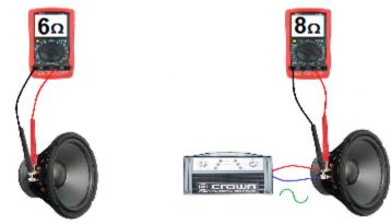
In the example above, we disconnected and tested an 8 ohm (8  $\Omega$ ) loudspeaker with a Multi-meter, and found it to be 6 ohms. This is the internal **Resistance** of the loudspeaker. Once an audio signal starts passing through, the internal resistance will rise to 8 ohms. This extra 2 ohms is called **Reactance** (the extra resistance caused by an audio signal passing through). The resulting 8 ohms is called the **Impedance** of the loudspeaker, which is what we refer to.
