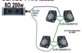
For those who like to play with wires, there is a configuration that involves 2 parallel circuits connected in series. The result is a perfectly balanced 8  $\Omega$  load, and the Power Amplifier will give out it's full 200watts. In this example each cabinet will get 50 watts of power.
